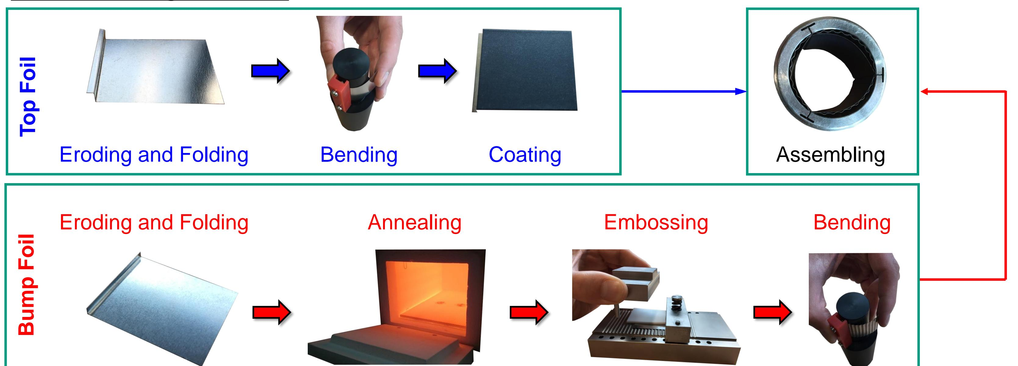
Thrust Bearing Manufacturing
